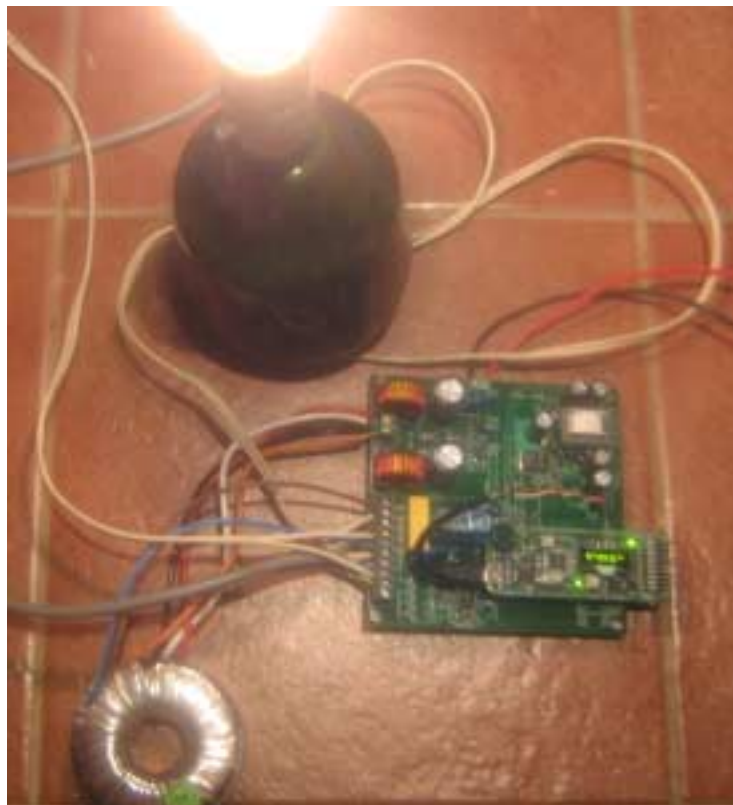
Photo 1. Solar UPS powering a 40W globe
